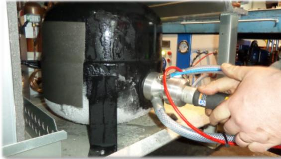
An operator is required to make the connection between the cooling device and the ATN 4 BK-PT. After the connection is established the machine takes over the control of the degassing cycle. The liquefied gas is conveyed into the designated tank. The cooling device will be vacuumed in order to reach the highest possible efficiency for the degassing. For safety reasons the drill-head can only be used in combination with the piercing device or the service connections of the cooling device.
